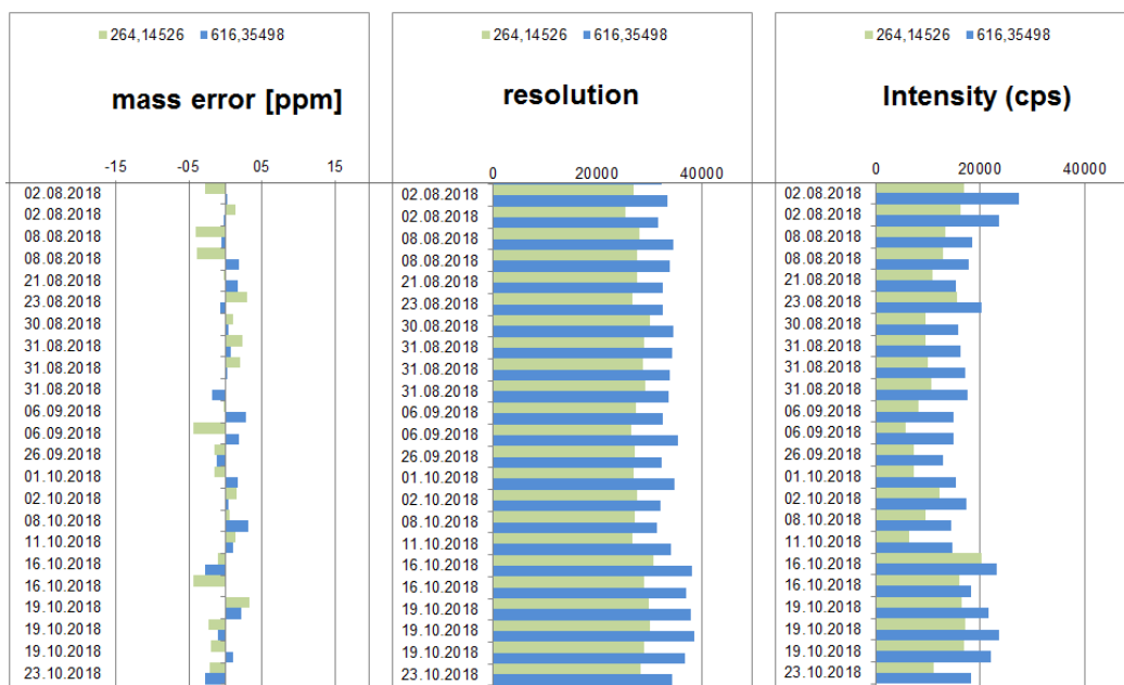
Figure E.3: Control charts to check MS performance via mass accuracy, resolving power (resolution) and sensitivity
